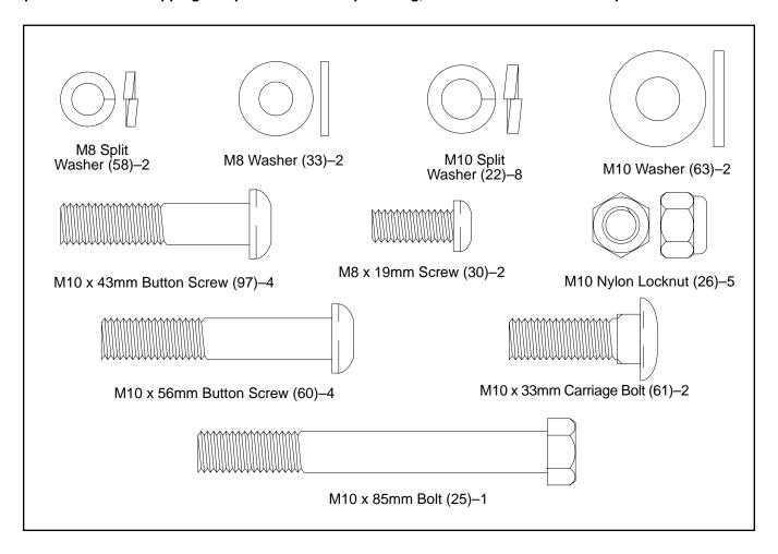
Identify the Rear Stabiliser (94), which has two Levelling Feet (99) threaded into it. Turn the Rear Stabiliser so the Levelling Feet are closest to the rear of the Frame (1) as shown. Attach the Rear Stabiliser to the Frame with the four M10 x 56mm Button Screws (60) and four M10 Split Washers (22).
